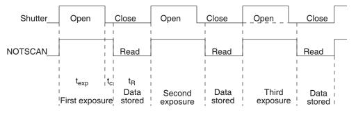
Figure 11. Free Run Timing Diagram
